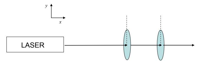
A student then turns off the laser. Then he/she rotates the first polarizer 45° clockwise and the second polarizer 45° counter-clockwise.
