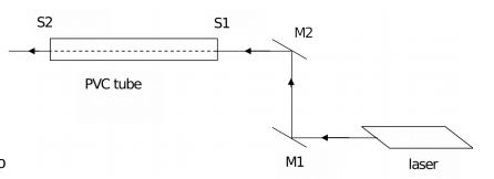
ways be parallel to the working (table) surface. The two mirrors allow you to change horizontal and vertical positioning accurately.
