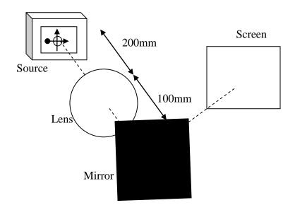
C) Suppose that the mirror were located 100 mm from the source and the lens located 100 mm from the mirror as shown in the diagram below. Once more the ray traveling along the optical axis reflects through a 90 degree angle. What is the distance from the lens to the screen? Draw the orientation of the image on the screen. Explain how you arrived at your answer.
