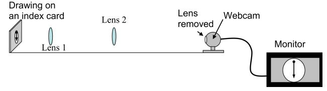
B. Where does the lens 1 form an image? Between lens 1 and lens 2, between lens 2 and the webcam, between lens 1 and the index card, behind the webcam, or behind the index card? How do you know?
