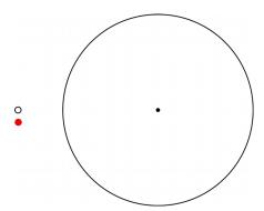
Place a fresh sheet of paper on the cork board. Then insert two source pins (use two different colors of pins) 1 cm apart into the board through the paper. Place a beaker filled to the height of the pin 2.5 cm inf front of the source pins and determine the image locations through triangulation for each pin. Did your observations agree with your prediction? Resolve any discrepancies.
